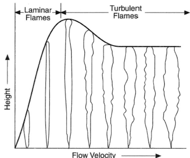
Fig. 1: Progressive Change in Flame Type with Increase in Jet velocity [1][2]
