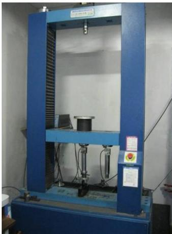
Fig. 10: Universal Testing Machine
