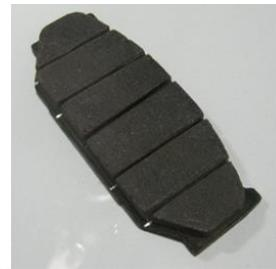
Fig. 1: Disc Brake shoe
