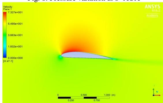
Fig. 9: Velocity at 4<sup>0</sup> AOA
