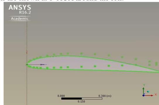
Fig. 3: Geometry of Airfoil created in ANSYS 16.2
