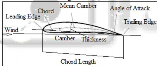
Fig. 1: Diagram of airfoil's geometry
