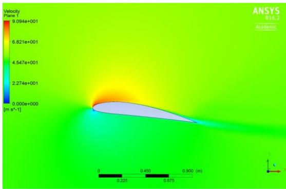
Fig. 10: Velocity at  $8^\circ$  AOA
