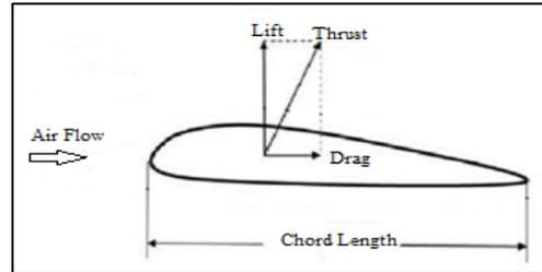
Fig. 2: Forces on a stationary airfoil in airflow
