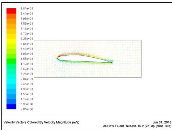
Fig. 6: Velocity Vectors around airfoil
