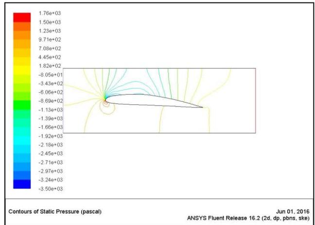
Fig. 2: Contours of Static Pressure
