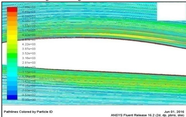
Fig. 5: Pathlines of Fluid Particles around aerofoil
