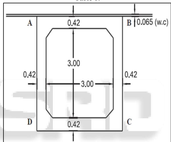
Fig. 1: Cross Section of Box Culvert
