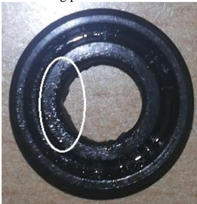
Fig. 5: Gas spring seal failure area
