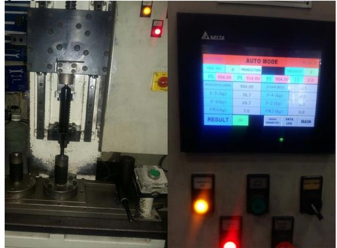
Fig. 4: Load cell arrangement and force measurement
