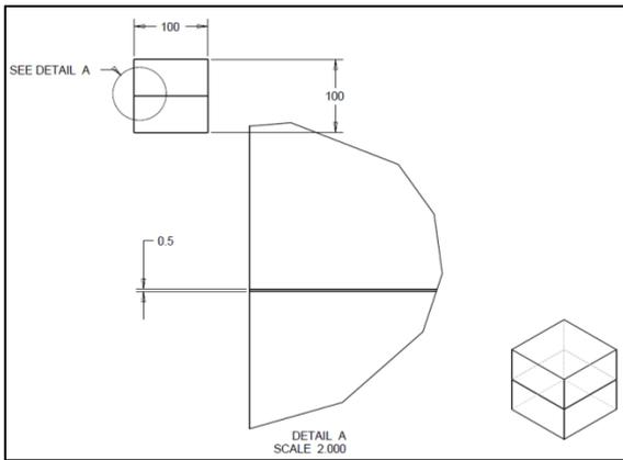
Fig. 2: Detailing of cube having 0.5% of other material
