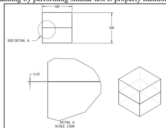
Fig. 1: Detailing of cube having 0.25% of other material
