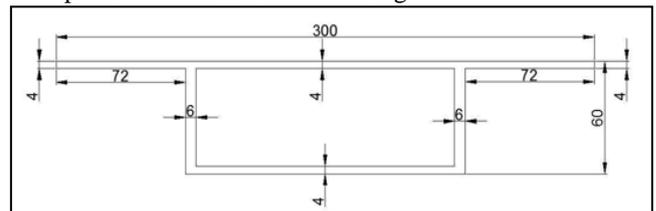
Fig. 4: Cross Section of Simply Supported Box Girder Bridge
