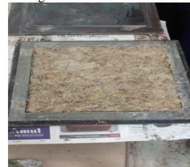
Fig. 4: Fibers poured in female die
