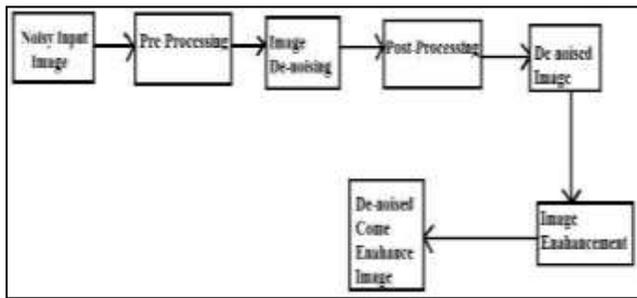
Fig. 3: Block diagram of Deep Sea Mine image De-noising & its Enhancement
