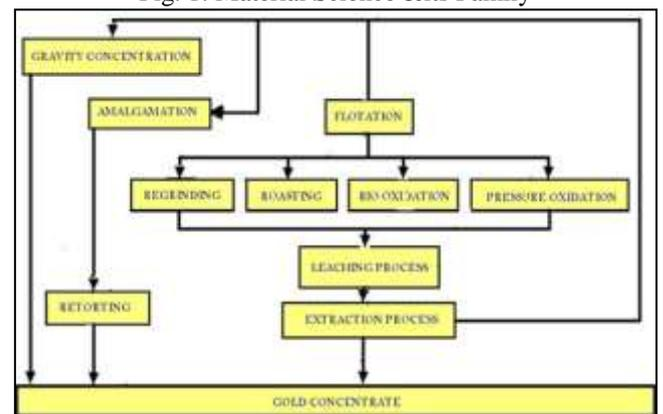
Fig. 2: Process of Extraction of Gold under Sea water
