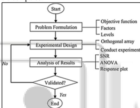
Fig. 1: Flow chart for optimization using Taguchi
