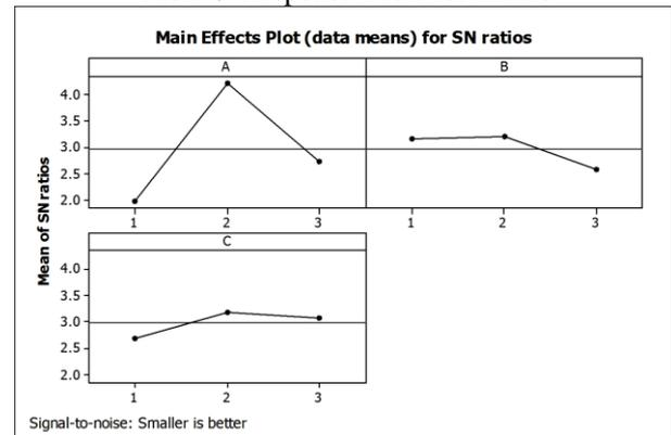
Fig. 2: Main effects for factors machining verse S/N ratio of surface roughness.
