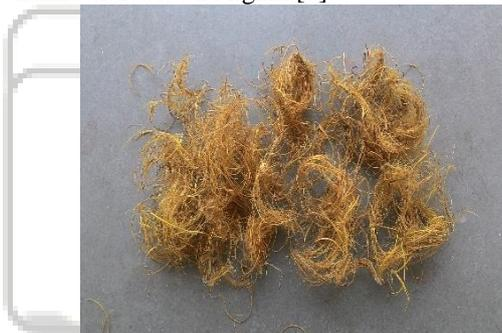
Fig. 1: Alkali treated Areca fiber
