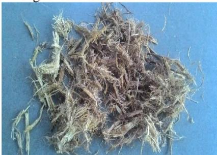
Fig. 2: Alkali treated Bagasse fiber
