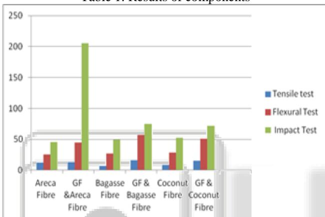
Fig. 7: Results of mechanical test
