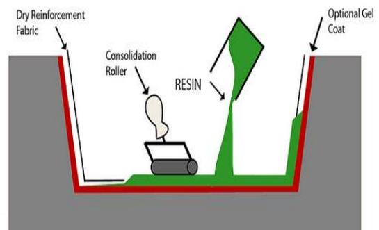
Fig. 5: Hand lay-Up method
