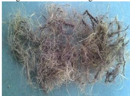
Fig. 3: Alkali treated Coco-nut fiber
