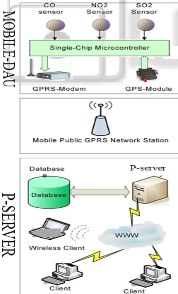
Fig. 1: System hardware basic building blocks.
