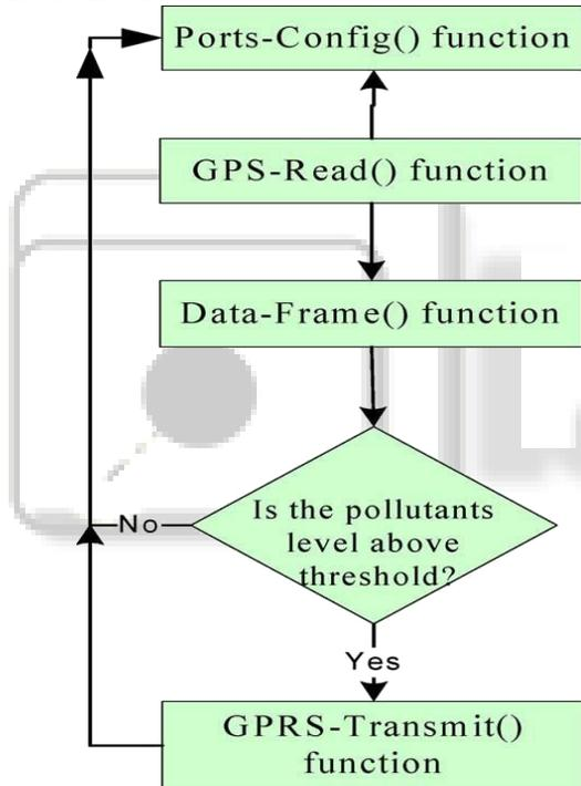
Fig. 2: Mobile- DAU Software Algorithm.
