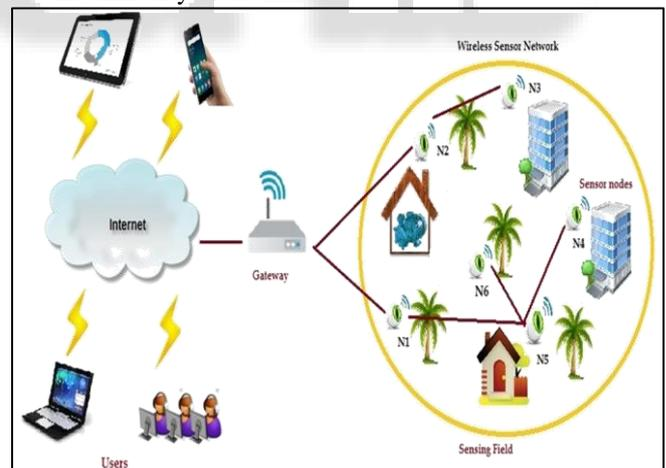
Fig. 1: Simple Wireless Sensor Network- WSN Architecture in a Small Campus
