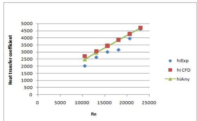
Fig. 5: Comparison between analytical, experimental and CFD heat transfer coefficients at various Reynolds numbers for plain tube.
