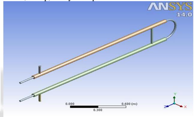
Fig. 1: Double pipe two pass heat exchanger model
