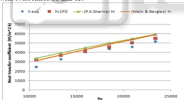
Fig. 8: Comparison between analytical, experimental and CFD heat transfer coefficients at various Reynolds numbers for twist ratio 20
