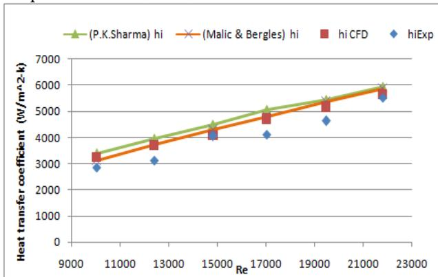
Fig. 7: Comparison between analytical, experimental and CFD heat transfer coefficients at various Reynolds numbers for twist ratio 15
