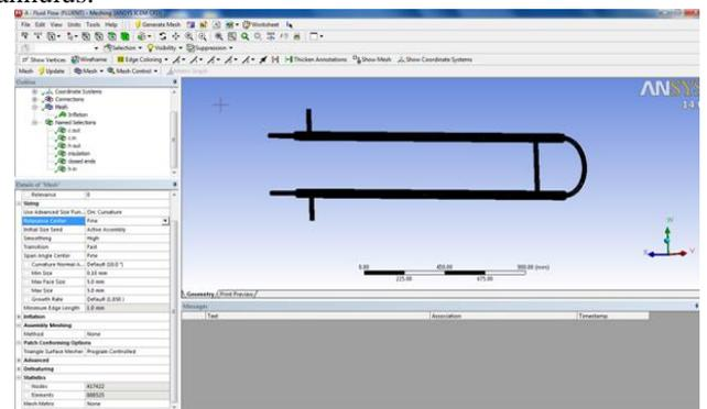
Fig. 2: Meshing of double pipe heat exchanger
