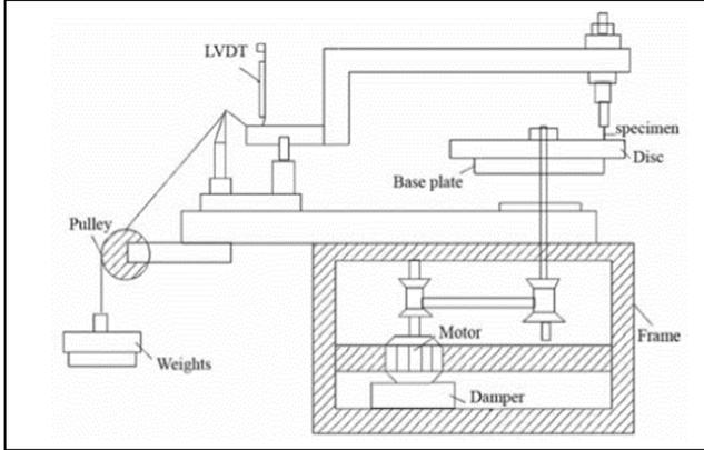
Fig. 1: Schematic Diagram of Pin on disc test rig
