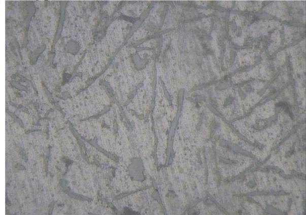
Fig. 2: (a) Microstructure of 3% SiC+5% Fly Ash at Magnification of  $\times 500$
