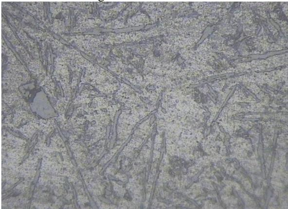
Fig. 2: (c) Microstructure of 6% SiC+5% Fly Ash at Magnification of  $\times 500$
