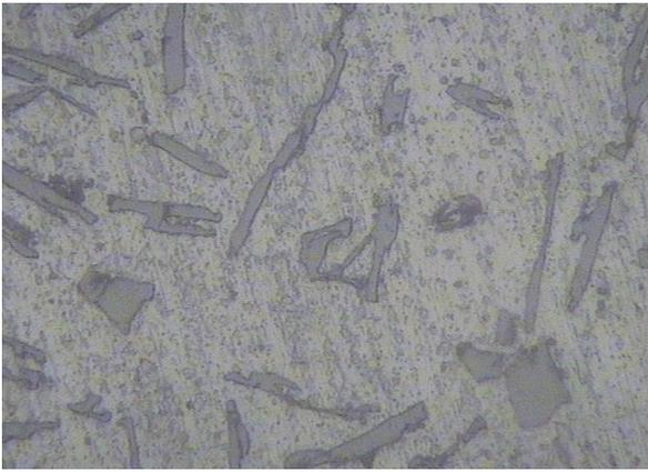
Fig. 2: (b) Microstructure of 3% SiC+5% Fly Ash at Magnification of  $\times 1000$
