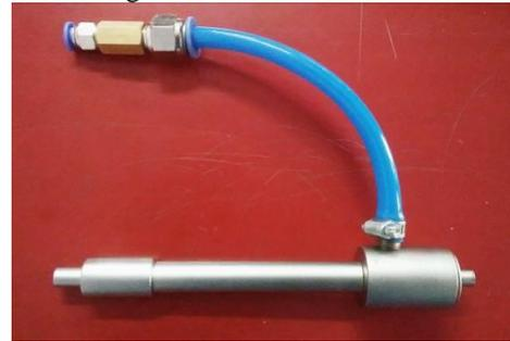
Fig. 10: Assembled vortex tube
