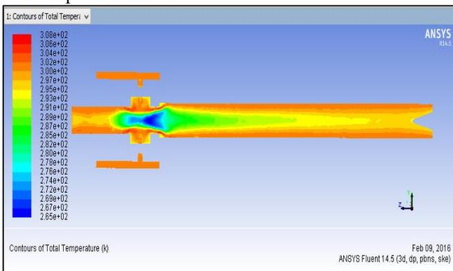
Fig. 2: Temperature contour at centre plane
