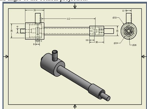
Fig. 4: Drawing of vortex tube
