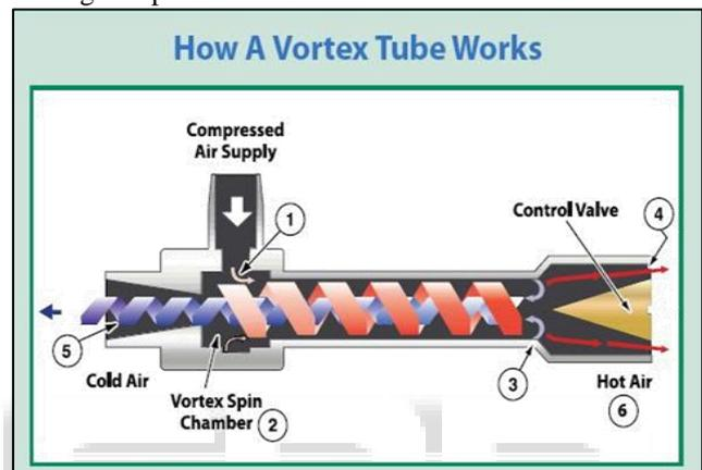
Fig. 1: Principle of Vortex tube [2]
