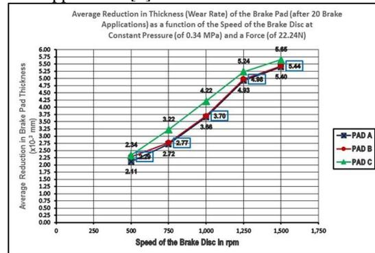
Fig. 4: Wear Rate of the Brake Pad as a function of the Speed of the Brake Disc
