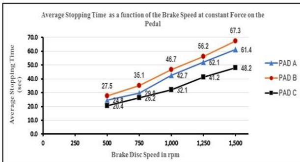
Fig. 5: Average Stopping Time as a function of the Brake Speed at constant Force on the Pedal
