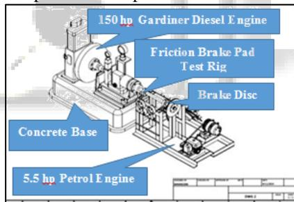
Fig. 1: Isometric view of the Diesel Engine and Brake Pad Test Rig Assembly
