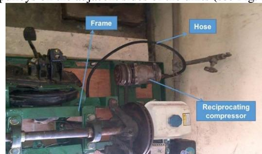
Fig. 3: Picture of the Compressor side of the Test Rig Assembly
