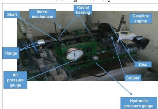
Fig. 2: Picture of the Friction Brake Pad Test Rig Assembly
