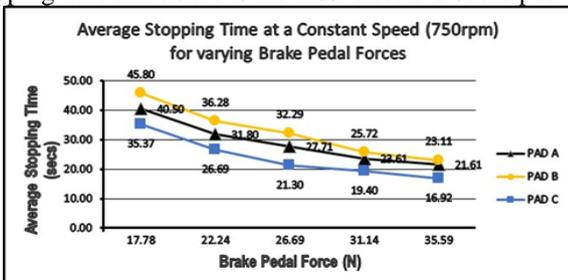
Fig. 6: Average Stopping Time of Brake Pad at constant speed (750 rpm) and for varying Brake Pedal forces.
