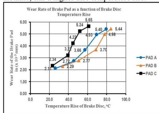
Fig. 7: Wear Rate of Brake Pad as a function of Brake Disc Temperature Rise
