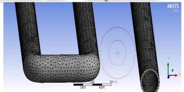
Fig. 7: Sectional view of the super heater tube after meshing
