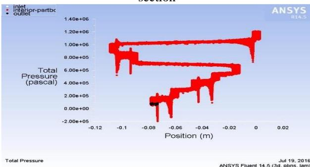
Fig. 12: Graph 3 The pressure variations throughout the tube
