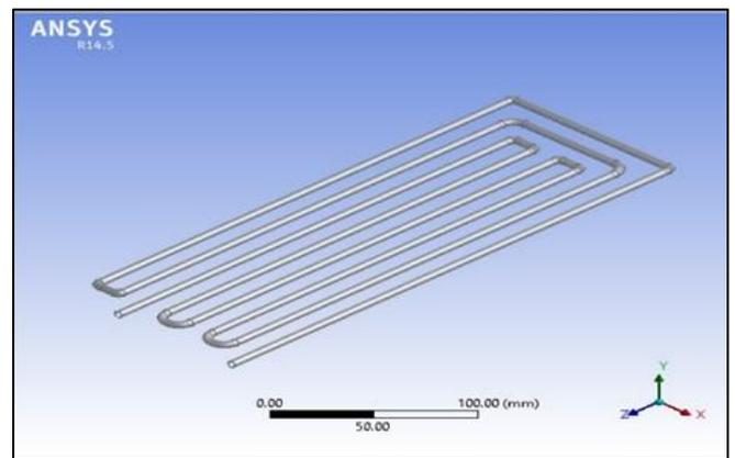
Fig. 5: 3d model created for analysis of super heater using ANSYS
