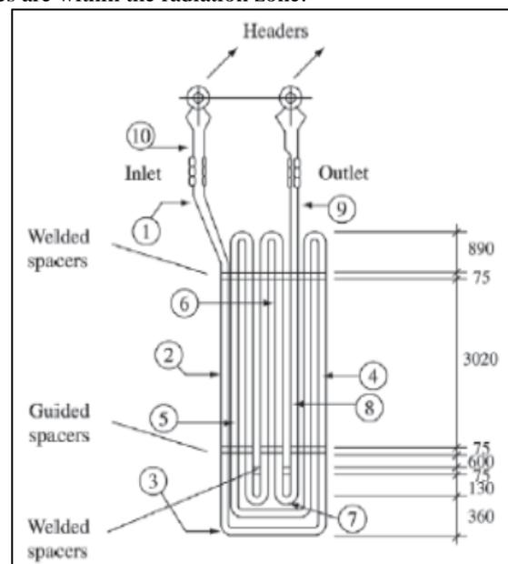
Fig. 3: Positions of the samples extracted from a primary super heater assembly
