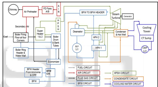
Fig. 2: Schematic diagram of a power plant
