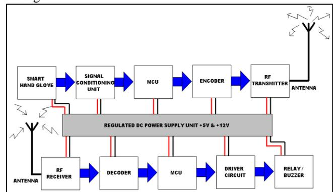
Fig. 1: Block Diagram of Implemented System
