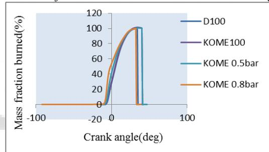
Fig. 8: variation of mass fraction burned with crank angle for diesel, biodiesel
