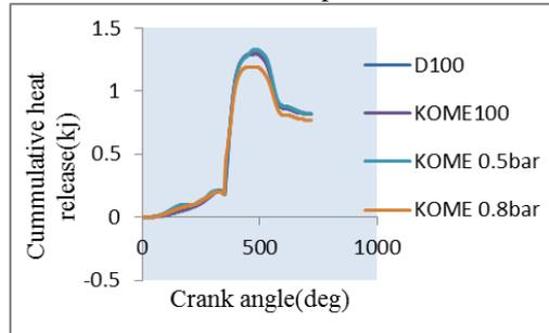
Fig. 7: Variation of cumulative heat release with respect to crank angle
