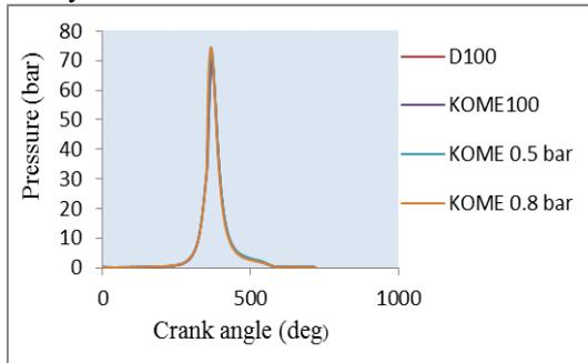
Fig. 5: Variation of Pressure with Crank Angle
