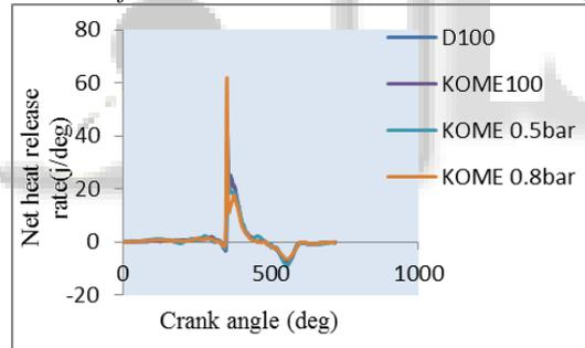
Fig. 6: Variation of Net Heat Release Rate with Crank Angle
