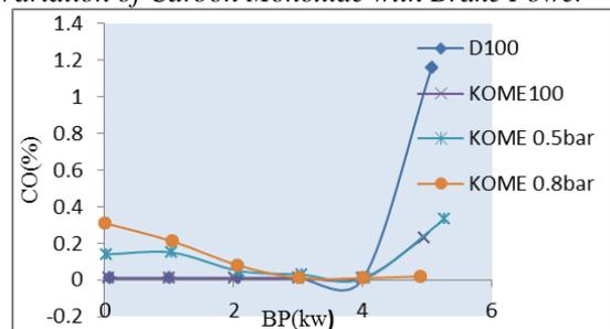
Fig. 9: Variation of carbon monoxide with brake power
