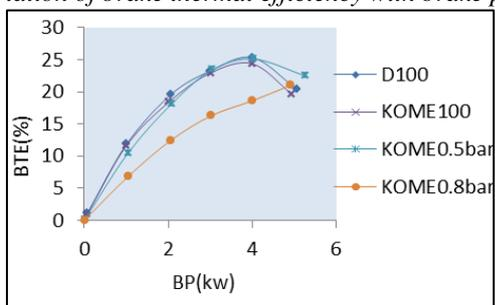
Fig. 3: Different Flow Rate of pressure between the brake power & brake thermal efficiency
