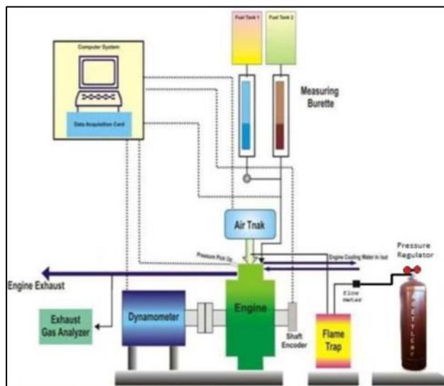
Fig. 1: Schematic of the experimental set up
