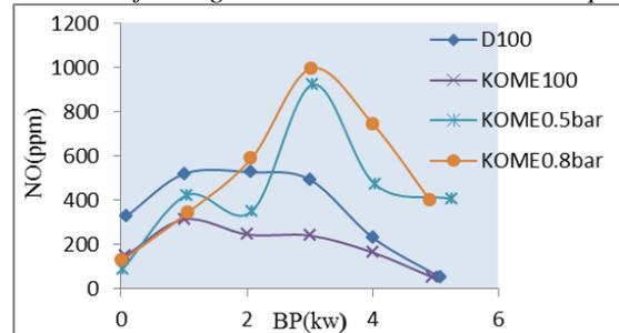
Fig. 11: Variation of nitrogen oxide emissions with brake power
