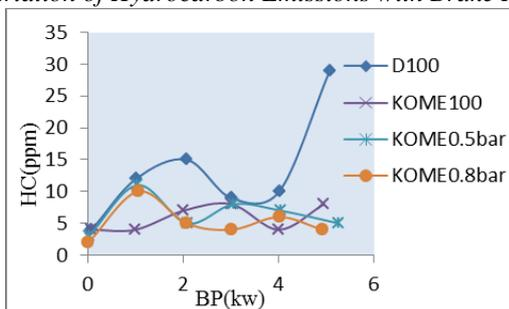
Fig. 11: Variation of Hydrocarbon Emissions with Brake Power
