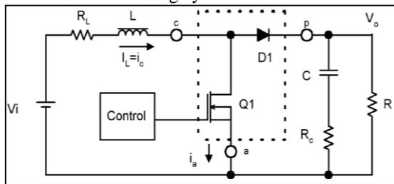
Fig 3. DC-DC converter
