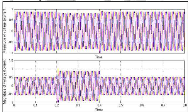
Fig. 7: 3-Phase Voltage and Current Waveform for Uncompensated System
