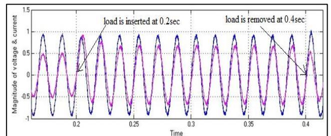
Fig. 12: 1 Phase Current and Voltage waveform when Load is Varied in the system
