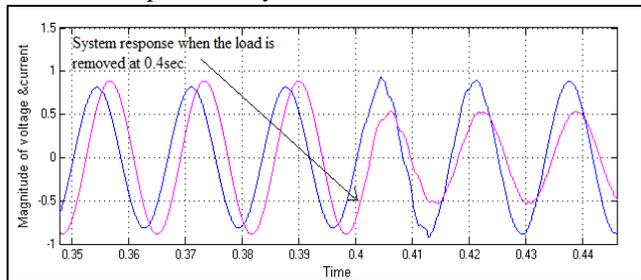
Fig. 6: Phase Voltage and Current Waveform for Uncompensated System when the load is removed
