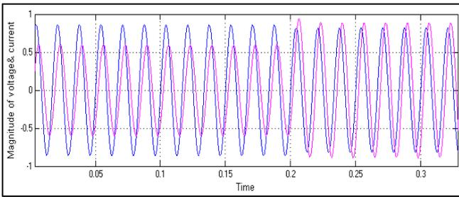
Fig. 4: Phase Voltage and Current Waveform for Uncompensated System
