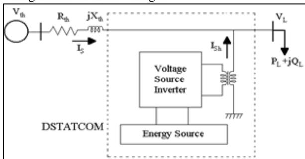
Fig. 1: Schematic Diagram of D-STATCOM
