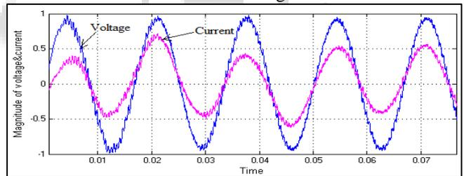
Fig. 11: Phase Current and Voltage waveform when the DSTATCOM is ON
