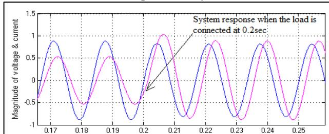
Fig. 5: Phase Voltage and Current Waveform for Uncompensated System when load is connected
