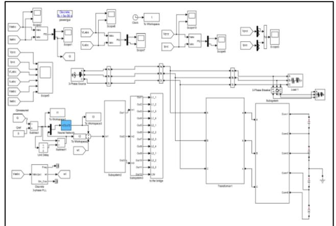
Fig. 9: Simulation Model of DSTATCOM based compensated system using ANN
