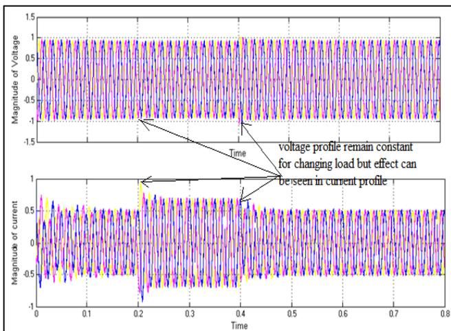
Fig. 13: 3-phase voltage and current waveform for DSTATCOM using ANN
