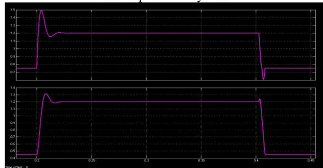
Fig. 8: Active and Reactive Power flow in uncompensated system
