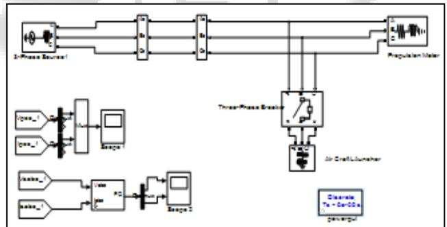
Fig. 3: Simulation Model of Uncompensated network
