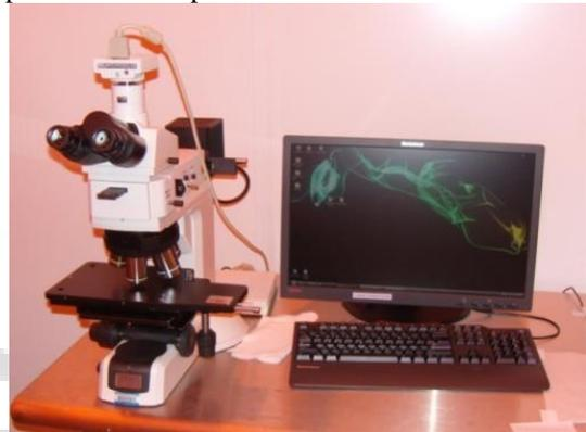
Fig. 4: Optical image analyzer
