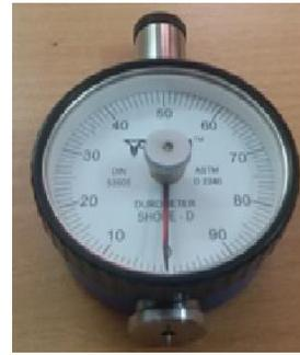
Fig. 3: Shore Durometer
