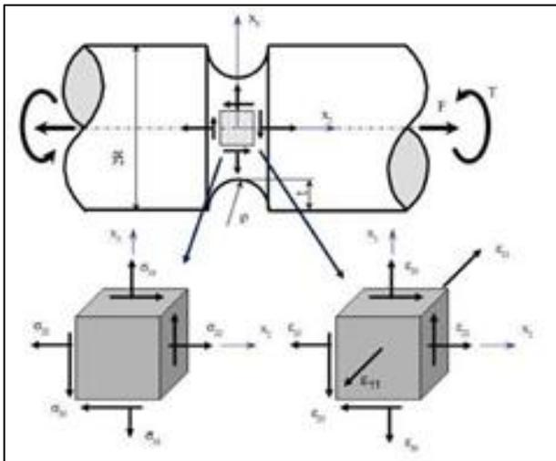
Fig. 4: Stress and strain state at a notch tip.
