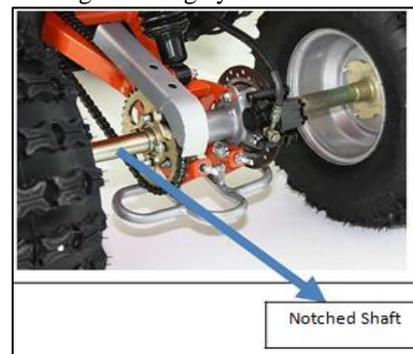
Fig. 2: Location of notched shaft in ATV
