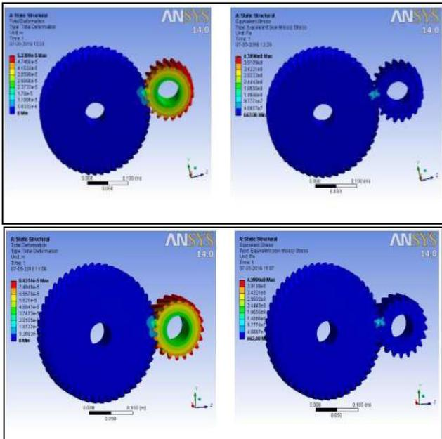
Fig. 6: For the Aluminum silicon carbide composite (Al-SiC) AT TORQUE = 400 N-m AT 3500 RPM
