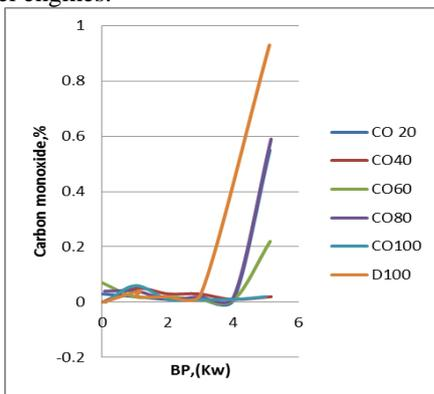
Fig. 9: Variations of Carbon monoxide Vs Brake power attetive in the blends.
