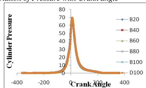
Fig. 11 Variation of Pressure with Crank angle
