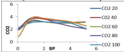
Fig. 8: Variations of Carbon dioxide Vs Brake power
