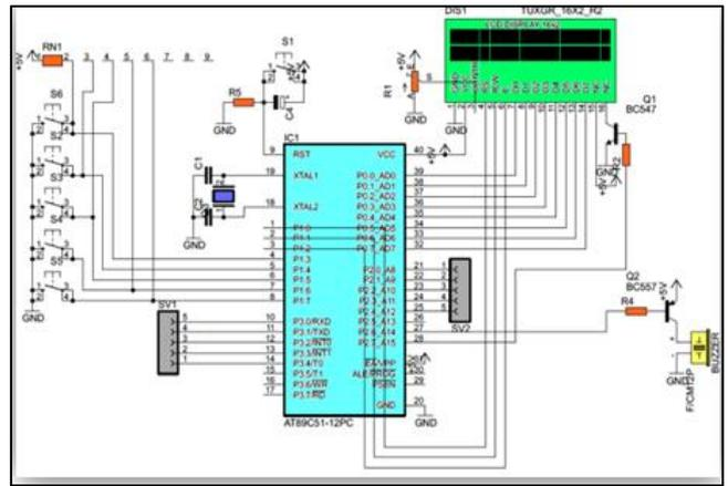
Fig. 3: Schematic Diagram of Ultrasonic Based Obstacle Detector System
