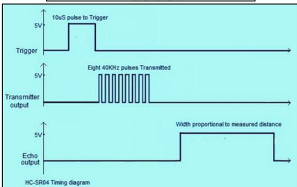
Fig. 2: Ultrasonic Sensor and its Functional Characteristics
