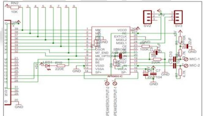
Fig. 4: Schematic Diagram of Proposed System
