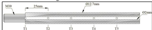
Fig. 2: Hollow Pin Fin with Inner Diameter = 2mm
