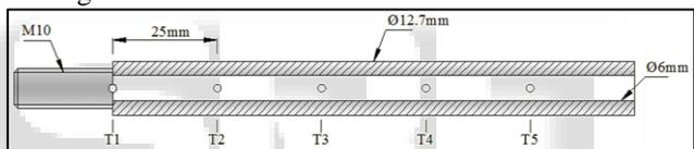
Fig. 3: Hollow Pin Fin with Inner Diameter = 6mm
