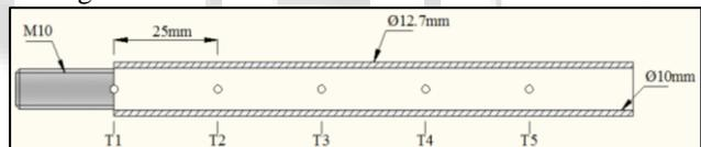
Fig. 4: Hollow Pin Fin with Inner Diameter = 10mm
