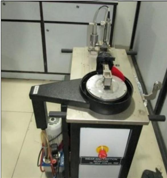
Fig. 1: Wear and friction monitor machine [16].
