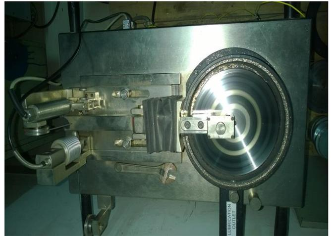
Fig. 2: pin on disc set up
