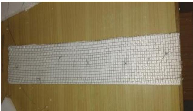
Fig.1: Thermocol with Wire Mesh
