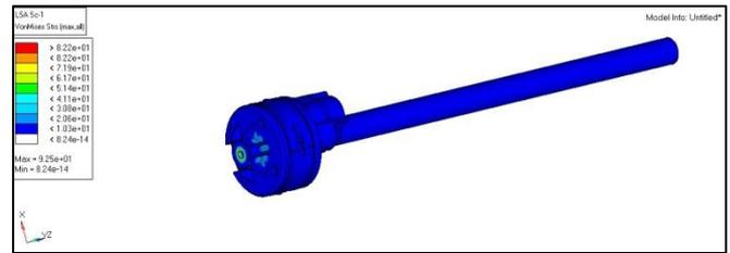
Fig. 11: VonMises stress: 92.5Mpa
