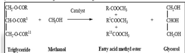
The production of biodiesel by transesterification of the oil generally occurs using the following steps:
