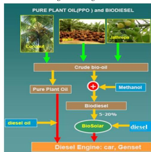
Fig. 1: Schematic diagram for producing bio diesel Biodiesel can be produced by esterification followed by trans esterification. The oils and fats are filtered and pre-processed to remove water and contaminants. If, free fatty acids are present, they can be removed or transformed into biodiesel using special pretreatment technologies. The pre-treated oils and fats are then mixed with an alcohol (usually
