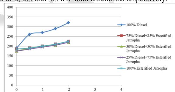
Fig. 10: Variation of brake power with exhaust gas temperature ( $T_{EX}$  Vs BP)
