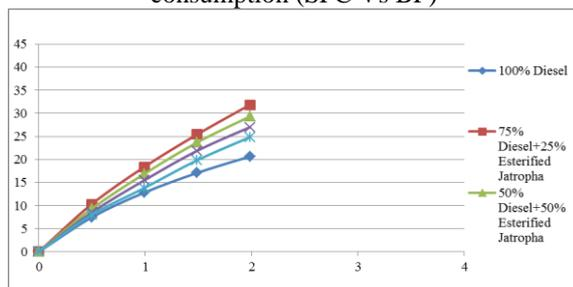
Fig. 9: Variation of brake power with brake thermal efficiency ( $\eta_{th}$  Vs BP)
