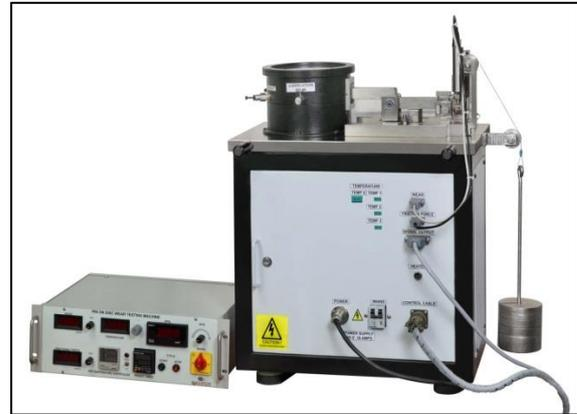
Fig. 1: Friction and Wear Tribotester (TR20LE)
