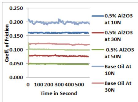
Fig. 3: Coefficient of friction of base oil with and without nanoparticles at 1% by wt. Al<sub>2</sub>O<sub>3</sub> concentration
