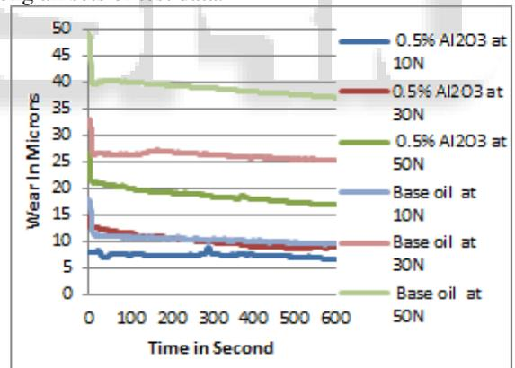
Fig. 2: Wear of base oil without nanoparticles and with 0.5 Wt. % Al<sub>2</sub>O<sub>3</sub> nano particles
