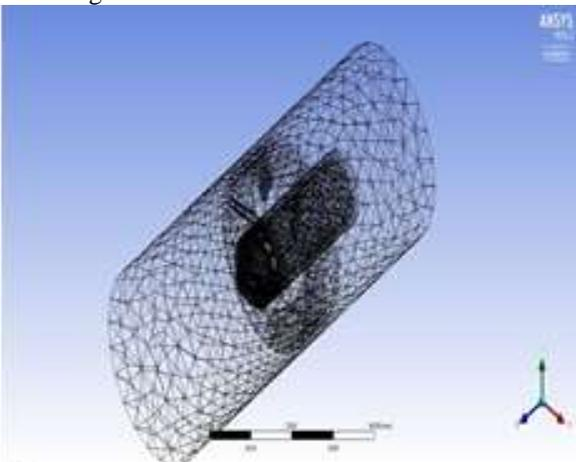
Fig. 3: Messing of the SWIRLER geometry
