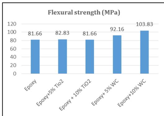
Fig. 5: Effect of fillers on flexural strength
