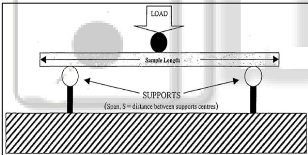
Fig. 1: 3 Point bending test
