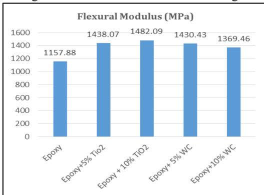
Fig. 5: Effect of fillers on flexural modulus
