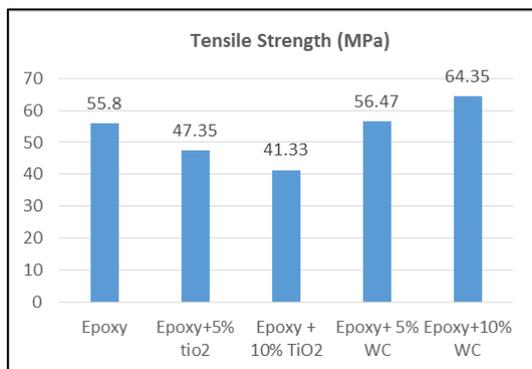
Fig. 2: Effect of fillers on tensile strength
