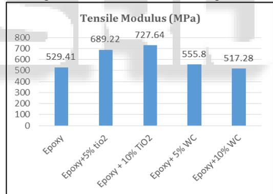
Fig. 4: Effect of fillers on tensile modulus
