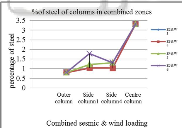
Fig. 6: Variation in reinforcement percentage in Columns for combined zones of seismic & wind.
