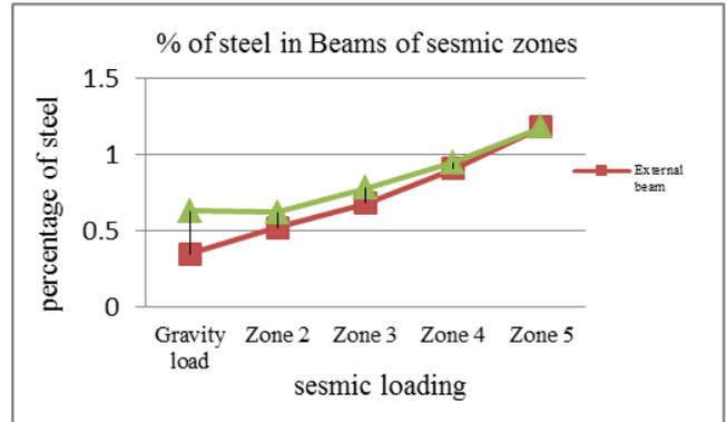
Fig. 8: Variation in reinforcement percentage in Beams for seismic zones
