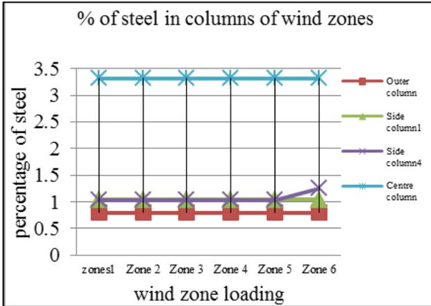
Fig. 5: Variation in reinforcement percentage in columns for wind zones.
