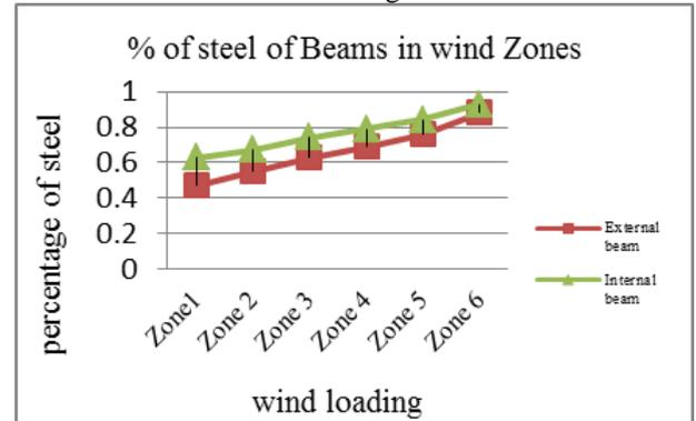
Fig. 8: Variation in reinforcement percentage in Beams for wind zones.
