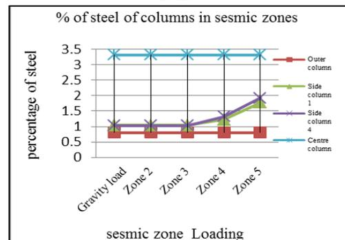
Fig. 4: Variation in reinforcement percentage in columns for seismic zones.
