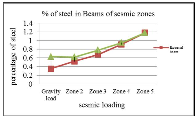
Fig. 7: Variation in reinforcement percentage in Beams for seismic zones
