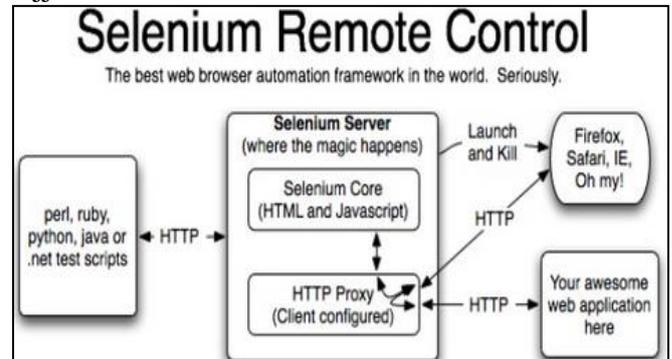
Fig. 1: Architecture of Selenium RC
