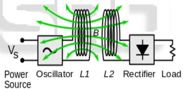
Fig. 2: Transformer Coupling
