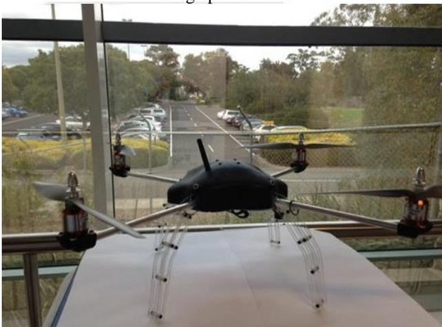
Fig. 7: A quadrotor for the power line inspection investigations.
