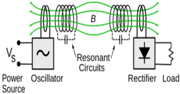
Fig. 4: Resonance Induction Coupling
