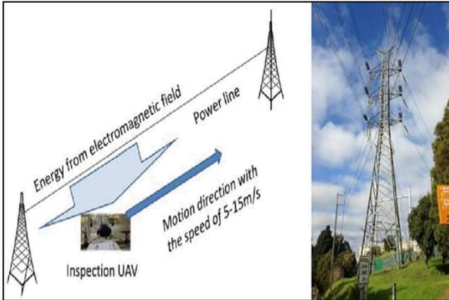
Fig. 6: Concept of powering UAV while inspecting high voltage power lines.
