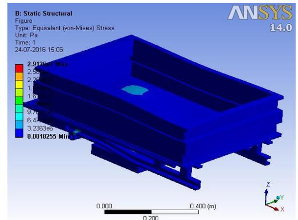
Fig. Maximum equivalent (von misses) stress is  $2.91 \times 10^2$  MPa.
