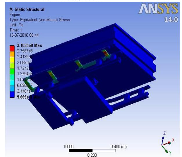
Fig. 8: Maximum equivalent (von misses) stress is  $3.10 \times 10^2$  MPa.
