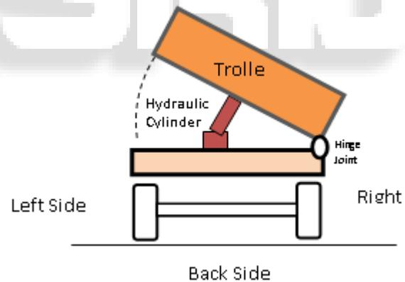
Fig. 3: Tilting diagram
