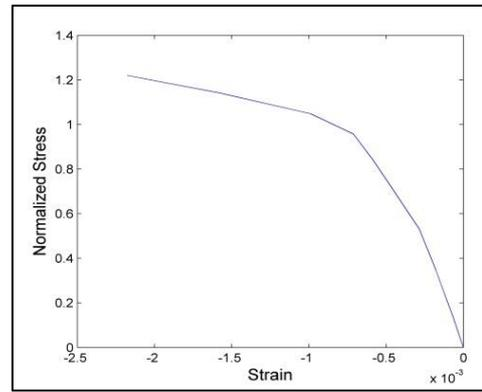
Fig. 3.3: Normalized stress v/s longitudinal strain curve for biaxial compression.
