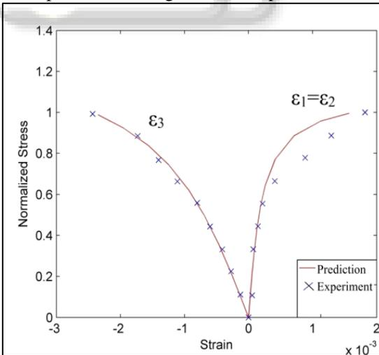
Fig. 4.3: Longitudinal and transverse strain for Group 3 of the specimen v/s longitudinal compressive stress
