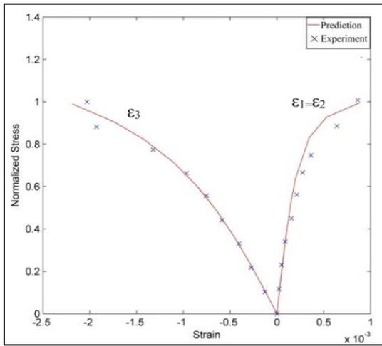
Fig. 4.1: Longitudinal and transverse strain for Group 1 of the specimen v/s longitudinal compressive stress
