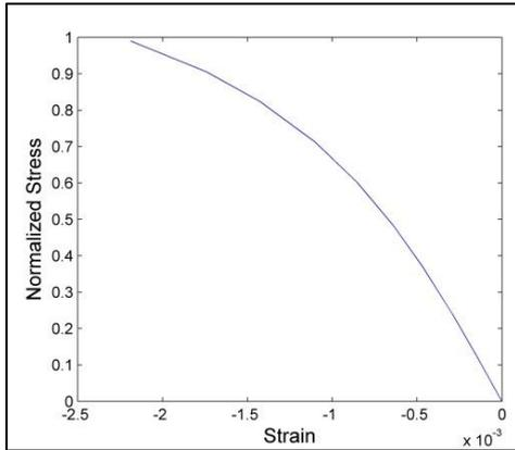
Fig. 3.1: Normalized stress v/s longitudinal strain curve for uniaxial compression.
