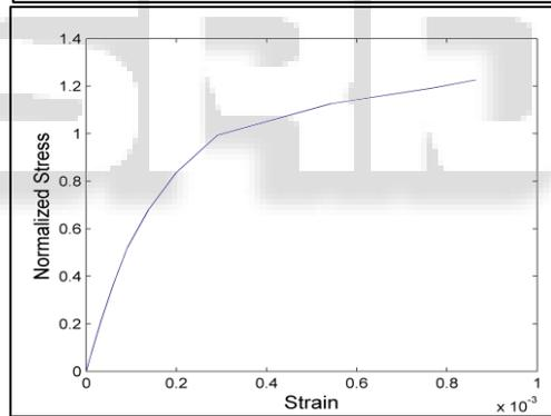
Fig. 3.4: Normalized stress v/s lateral strain curve obtain as for biaxial compression
