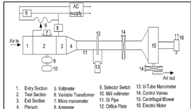
Fig. 4: Circuit Diagram
