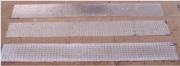
Fig. 2: Rough plate of different Pitches
