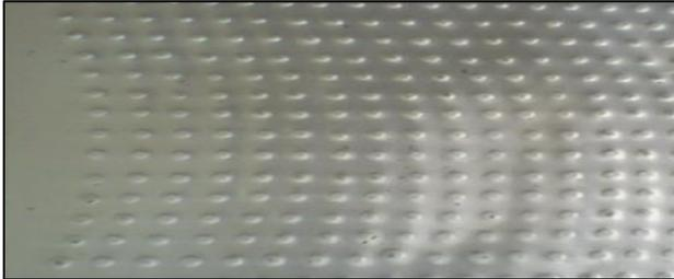
Fig. 3: Protruded roughness geometry
