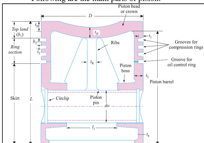
Fig. 1: Piston Components for I.C. engine
