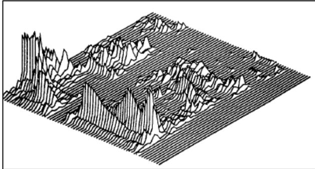
Fig. 4: Short-time spectrum using bias removal, half-wave rectification, residual noise reduction, and non speech signal attenuation (helicopter speech).
