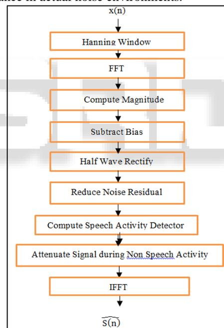
Fig. 1: Block diagram Suppression of Acoustic Noise in Speech Using Spectral Subtraction.
