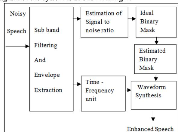
Fig. 4: System Block Diagram for speech enhancement using Ideal Binary Mask
