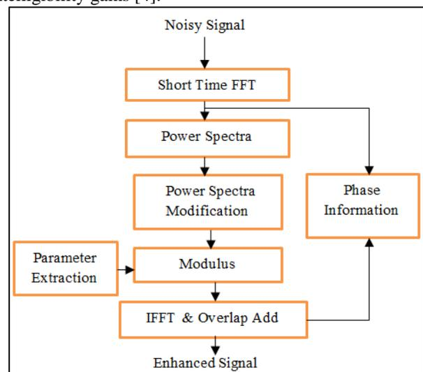
Fig. 5: General block diagram for the ANS technique
