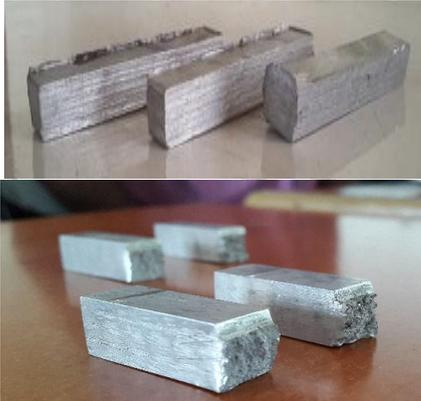
Fig. 4: Charpy test piece
