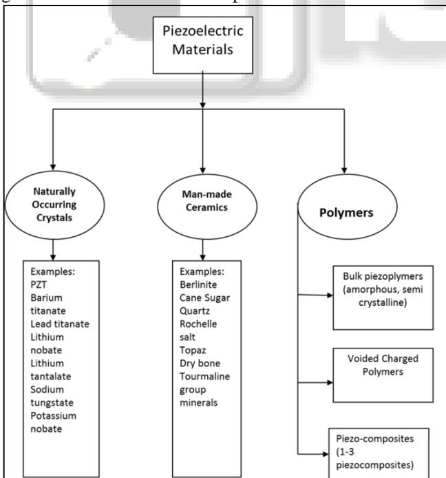
Fig. 1: Classification of Piezoelectric Materials
