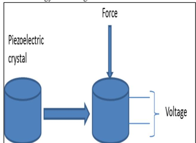
Fig. 2: Principle of direct piezoelectric effect Tanvi et al.(2010)
