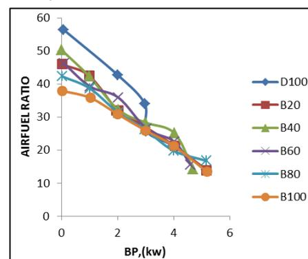
Fig. 12: Variation of Air fuel ratio with Brake power
