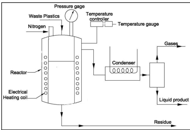
Fig. 8: Oil extraction plant for waste plastics
