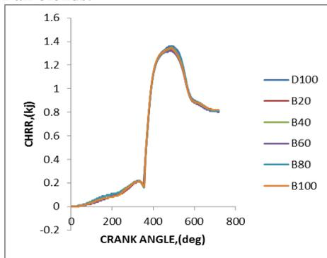
Fig. 21: Variation of Cumulative heat release rate with Crank angle
