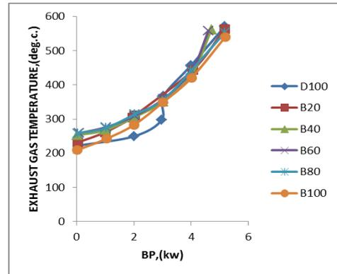
Fig. 15: Variation of Exhaust Gas Temperature with Brake power
