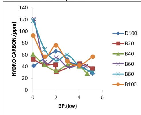
Fig. 16: Variations of Unburnt Hydrocarbon Vs Brake power
