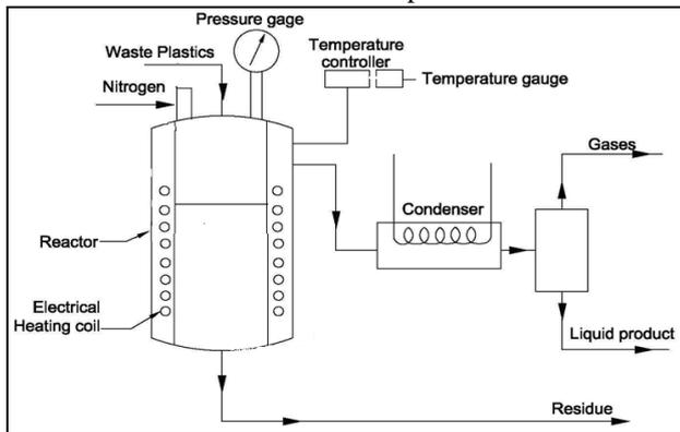
Fig. 5: Oil extraction plant for waste plastics
