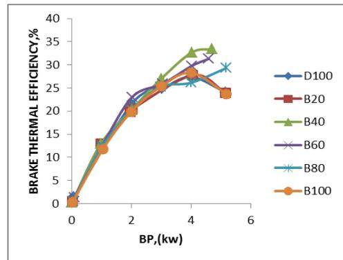
Fig. 10: Variation of Brake thermal efficiency with Brake power
