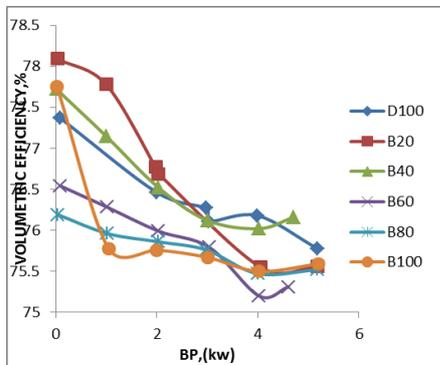
Fig. 14: Variation of Volumetric efficiency with Brake power
