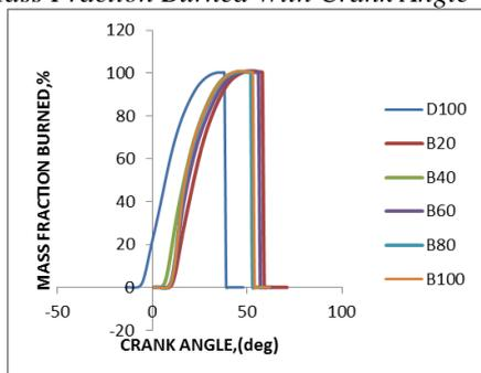
Fig. 23: Variation of net mass fraction burned with Crank angle
