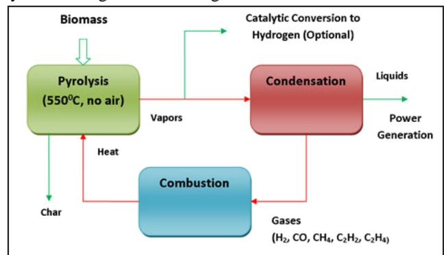
Fig. 7: Pyrolytic Process
