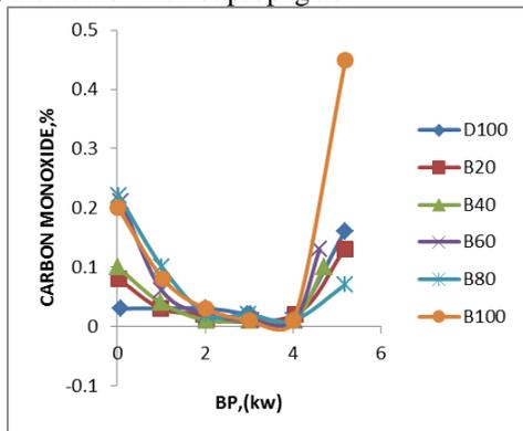
Fig. 18: Variations of Carbon monoxide Vs Brake power
