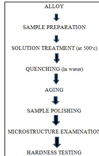
Fig. 3: Flowchart of Precipitation Hardening
