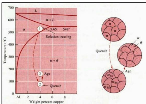
Fig. 2: The aluminum rich end of the Al-Cu phase diagram showing the three steps in the age-hardening heat treatment and the microstructures that are produced.
