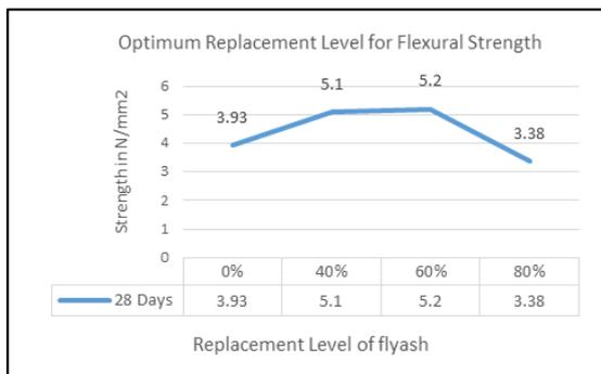
Fig. 6: Optimum Replacement Level for Flexural Strength.
