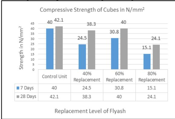
Fig. 1: Compressive strength of concrete at various replacement levels
