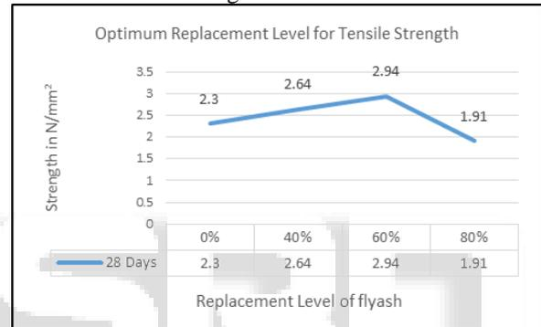
Fig. 4: Optimum Replacement Level for Tensile Strength.
