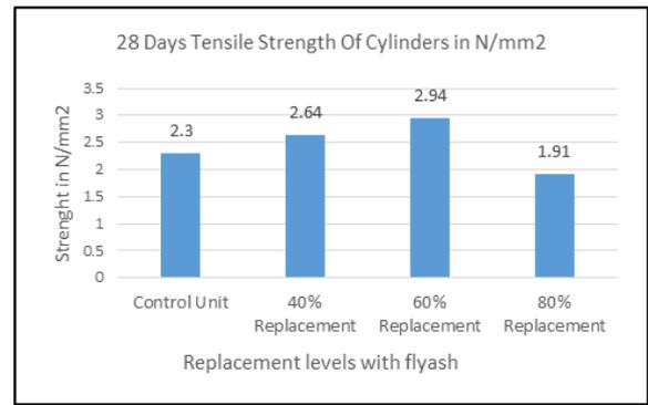
Fig. 3: 28 Days Tensile Strength of Cylinders at various replacement levels.
