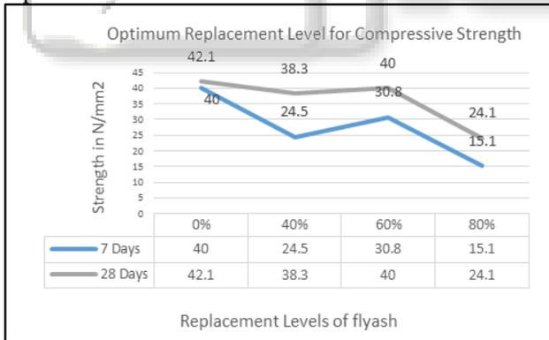
Fig. 2: Optimum replacement levels for compressive strength
