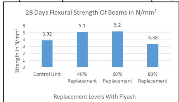
Fig 5: 28 Days Flexural Strength of Beams in various replacement levels.
