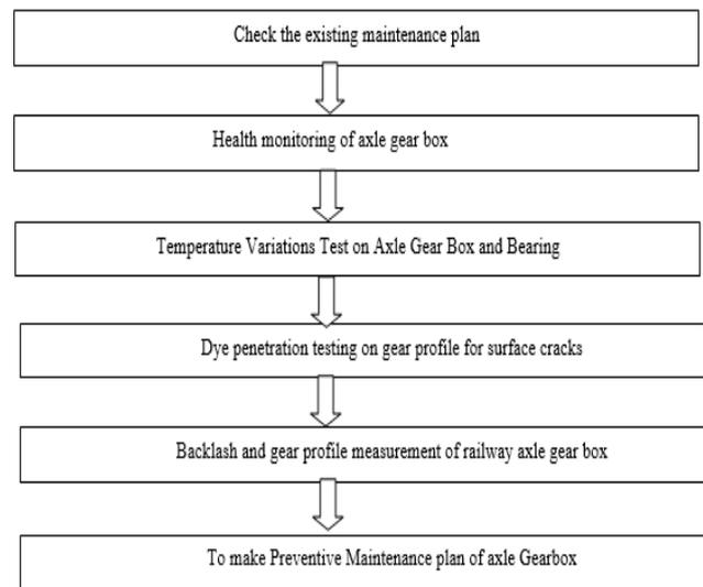
Fig. 2: Methodology for analysis of gear profile and backlash of railway axle gear box
