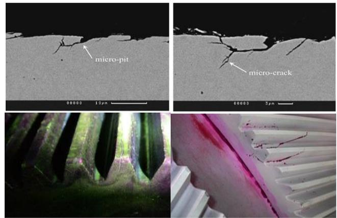
Fig. 4: Cracks on gear profile
