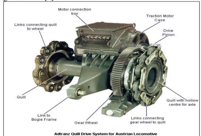
Fig. 1: Diagram of DC suspended traction motor and bearing arrangement [6]
